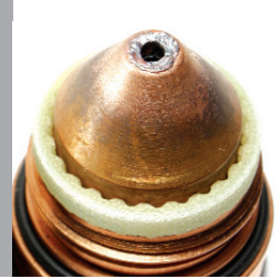
Fully-used OEM nozzle after 1,100 starts
