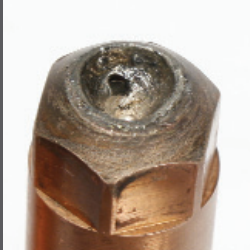
Fully-used OEM electrode after 1,100 starts
