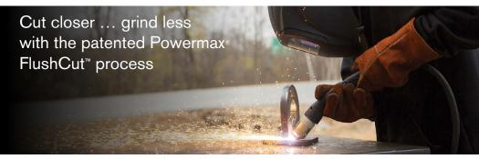
The FlushCut process for cutting/removing attachments, lugs and pad eyes leaves less than 3/16" (5 mm) of residual material behind. This significantly reduces grinding time and increases the ability of the attachment, lug or pad eye to be reused.
